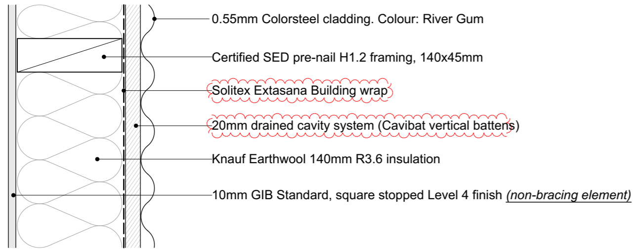
TYPICAL EXTERNAL WALLS (140mm shown here)
